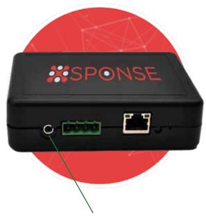
X-Guardian monitors resistance on the audio output in real-time to provide immediate notifications in the event of device tampering or PA system failure.
